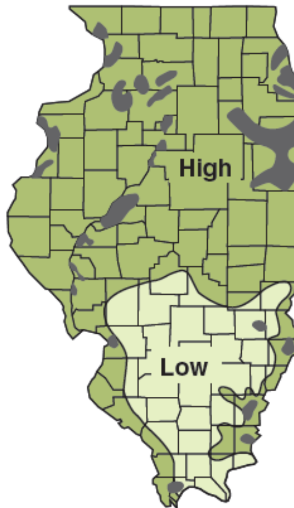
Figure 8.7. Cation-exchange capacity of Illinois soils. The darkest areas are sands with low capacity.
